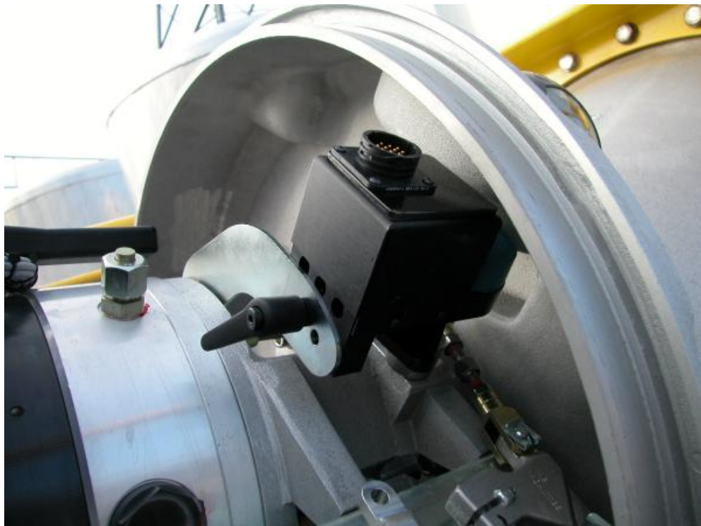
Rotary Transducer on ABB HMB Mechanism
