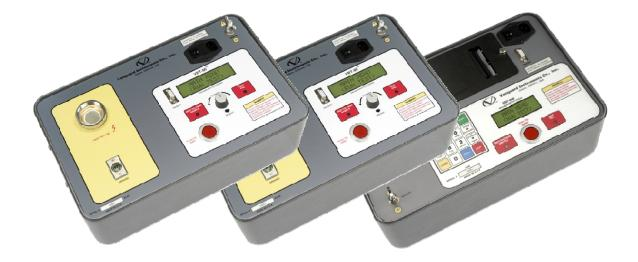
The VBT-60, VBT-80, and VBT-80P are light-weight DC vacuum bottle testers. The VBT tests the vacuum bottle integrity by applying a DC voltage across the bottle under test. A simple "PASS" or "FAIL" message indicates the condition of the bottle after each test. The VBT is field-portable, rugged, and is easily operated by first-time users having a minimum of training. It features a "Turn-then-Press" control knob for entering test parameters and control functions.
