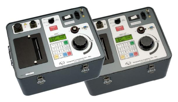
The EZCT is a microprocessor-based, current-transformer test set. This rugged and portable test set can perform the current transformer (CT) excitation, CT current-ratio, and winding polarity tests. Current transformers can be tested in their field-mounted configuration, eliminating the need to remove bushings or current transformers from the host equipment. The EZCT is capable of outputting 50 Vac at 2A and 200 Vac at 2A.
