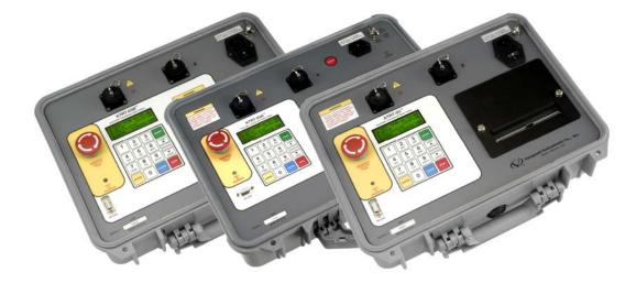
The ATRT-03 line is Vanguard's second generation family of microprocessor-based, automatic, three phase, transformer turns-ratio testers. The ATRT-03 line consists of the following three models:
