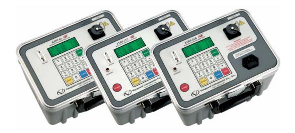
The ATRT-01 S2 is Vanguard's third-generation micro-processor-based, single-phase, automatic, transformer-turns-ratio tester. This portable test equipment is offered in three models: the ATRT-01 S2, ATRT-01B S2, and ATRT-01D S2. The ATRT-01 S2 is ac-line powered; the ATRT-01B S2 is ac-line or rechargeable-battery powered, and the ATRT-01D S2 is powered by six D-cells.
