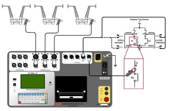
Figure 1. Typical Connection Diagram for an On-line Test
