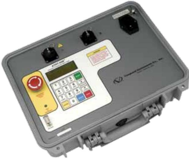
The ATRT-03B can perform a specific test for each transformer type (such as single phase, delta to Y, Y to delta, delta to delta, or Y to Y) without the need to switch test hookup cables. Also, the unit's automatic transformer phase detection feature can detect different transformer vector diagrams. The ATRT-03B can automatically detect and test 67 transformer types defined by ANSI, CEI/IEC and Australian standards.
