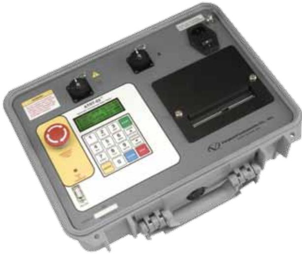
The ATRT-03 is Vanguard's second generation, microprocessor-based, automatic, three phase, transformer turns-ratio tester. This lightweight, portable unit is designed for testing transformers at utility power substations.
