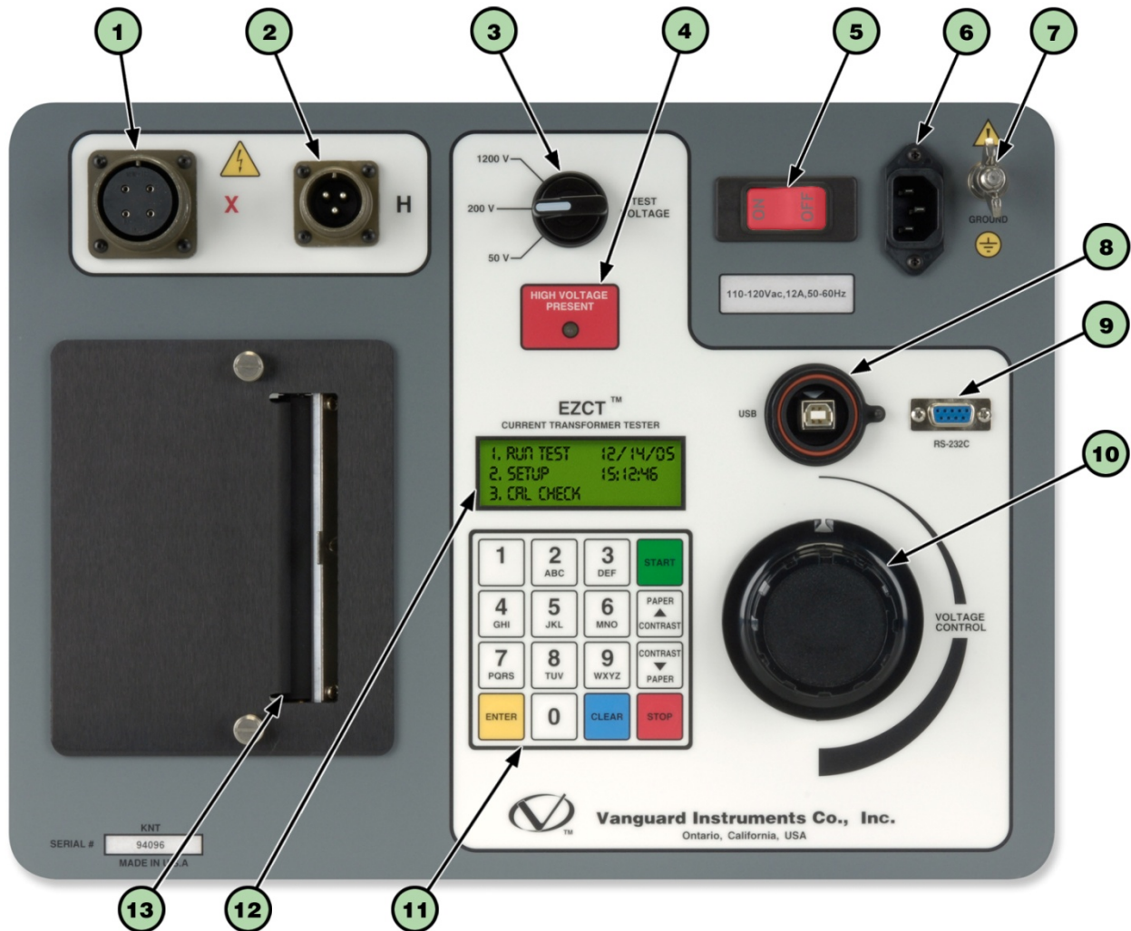
Figure 1. EZCT/EZCT-10 Controls and Indicators
